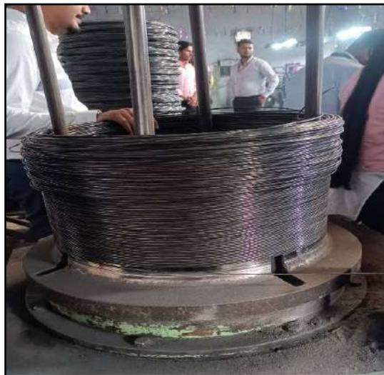
**Iron Coil for Converting into Electrode**
